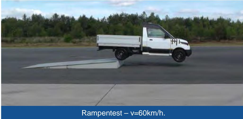
Rampentest –  $v=60\text{km/h}$ .
